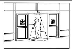
**Figure 1** Walk through Detection Zone
