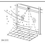
Sensor is exposed to: Steam, Exhaust Fume, Insects, Heavy Rain, Heavy Snow.
