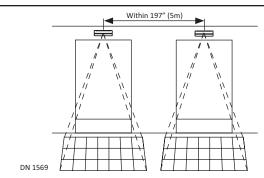
Multiple Sensors installed close together, or facing each other.
