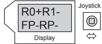
Only (1) Relay PCB Board (R0) has been installed
