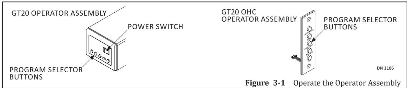
**Figure 3-1** Operate the Operator Assembly
