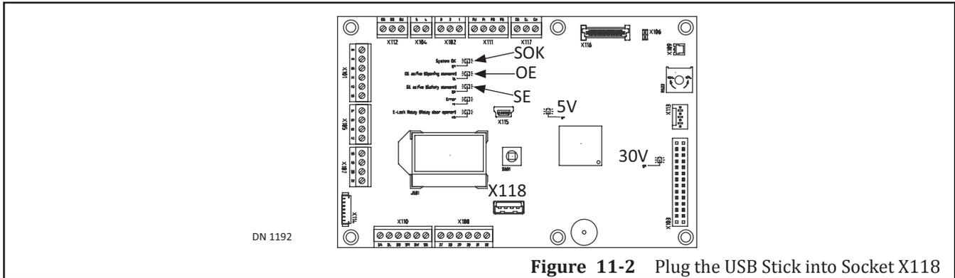
**Figure 11-2** Plug the USB Stick into Socket X118
