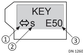
Swing door: in Night Mode; is opening; and communicating to a Slave door; (1) System Error
